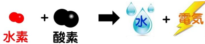
SOFC(solid oxide fuel cell)
